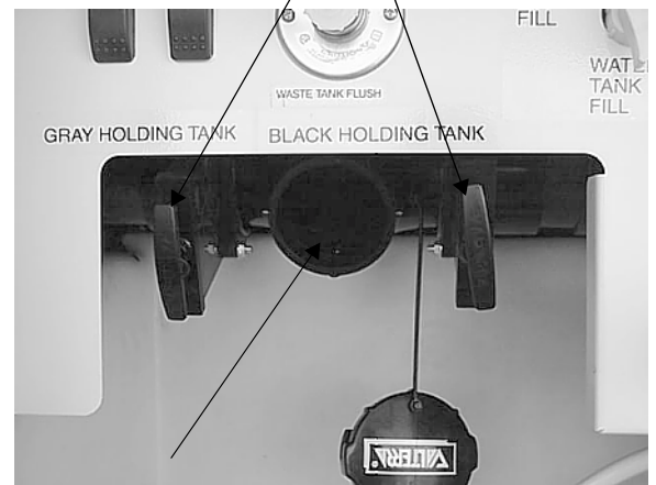
Sewage Dump Hose Outlet
