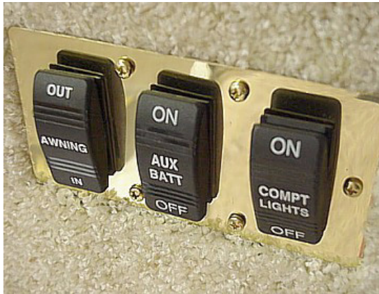
Aux. Batt. Disconnect Switch in Entrance Stepwell
