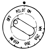
Oven Control Knob in “PILOT ON” position
