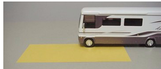
Weighing Left Front ‘Corner’
