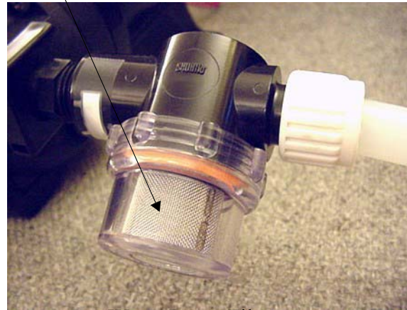
Water Pump Filter
