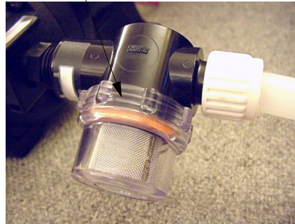
Water Pump Strainer
