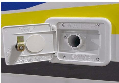
Water Tank Gravity Fill (typical)
