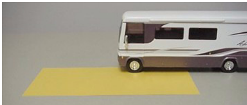
Weighing Left Front ‘Corner’
