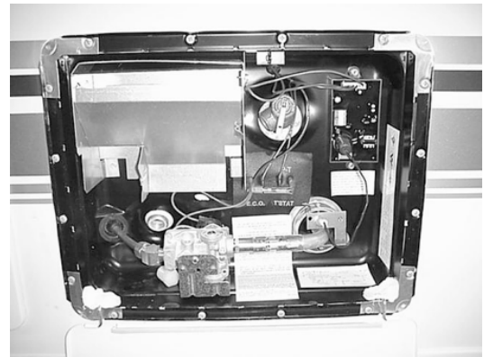
Water Heater Exterior Service Access
