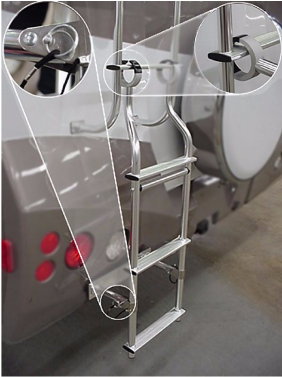
Roof Ladder Extension (typical)
