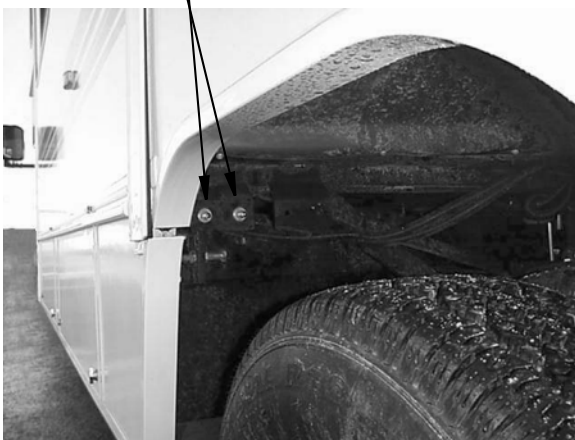
Rear Air Spring Valves located inside left rear wheel well
