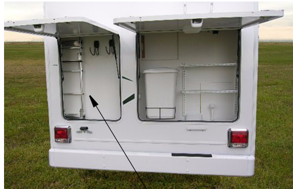
Roof Ladder Extension Storage
