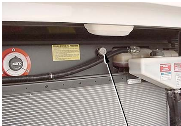
Diagnostic plug on rear engine compartment shroud
