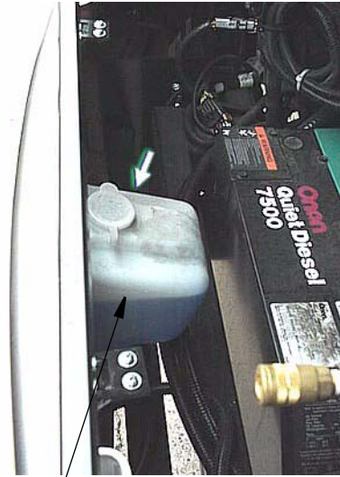
Windshield Washer Reservoir behind front "hood" panel.
