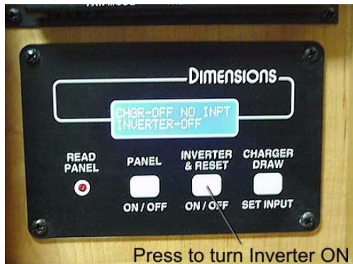
Inverter/Charger Control Panel
