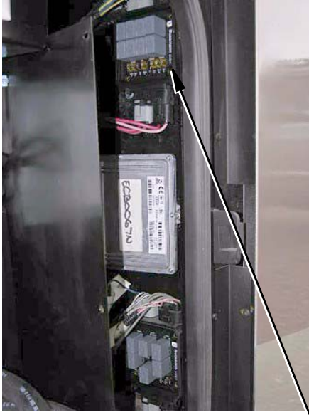
Towing Package fuses are on fuse block
