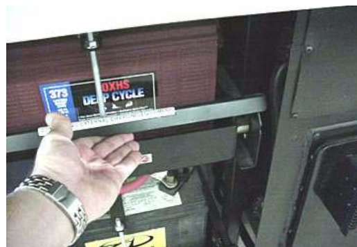
Lift Battery Tray Retainer Latches
