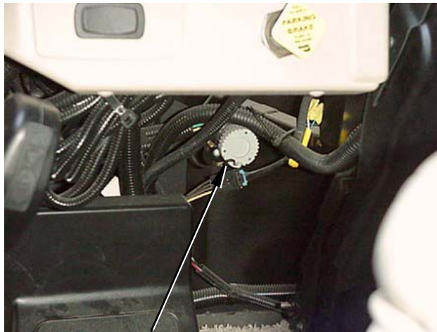
Diagnostic plug on steering column support beneath left side of dash
