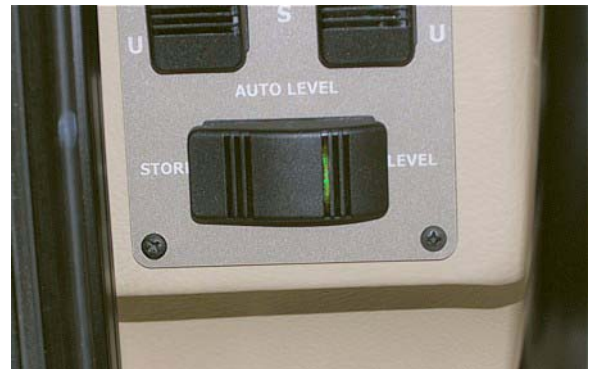
Auto Level Switch inside Entrance Door
