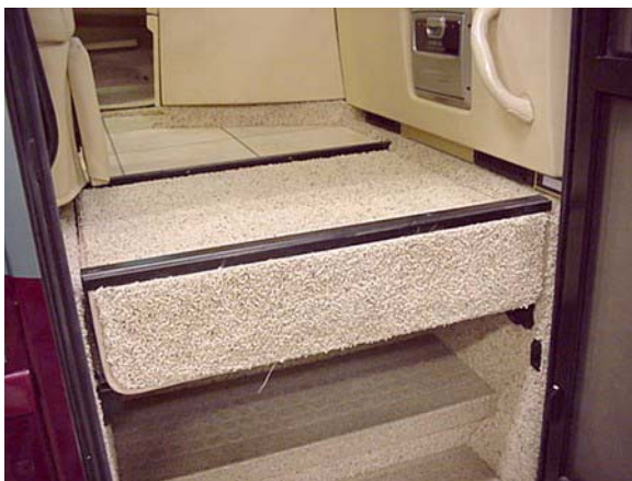
Step Cover shown in extended position (typical)
