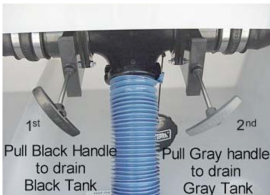
Holding Tank Dump Valves (Typical)
