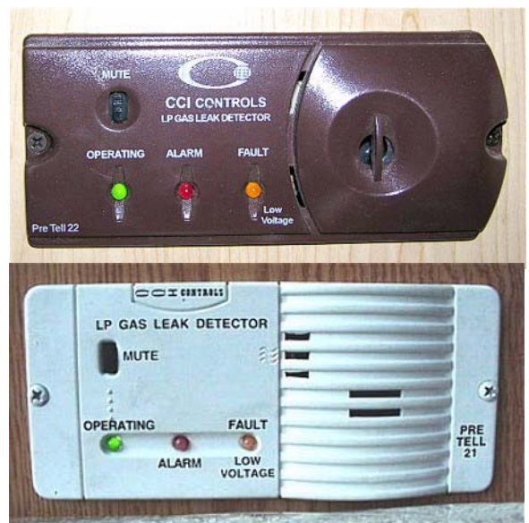
Propane Gas Leak Detectors (typical)
