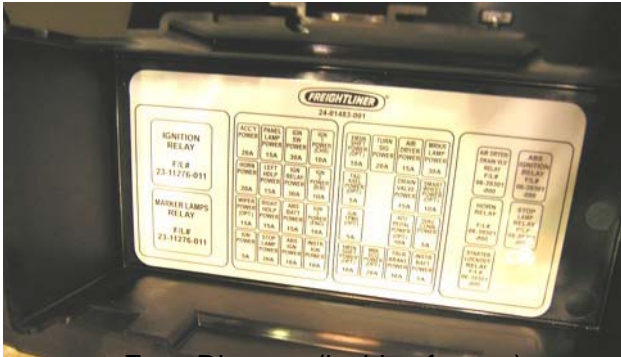
Fuse Diagram (inside of cover)
