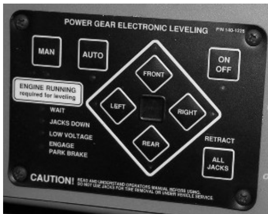
Leveling System Control Panel
