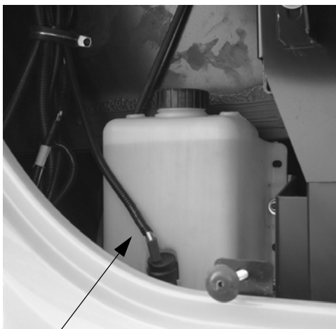
Windshield Washer Reservoir (behind front hood panel)
