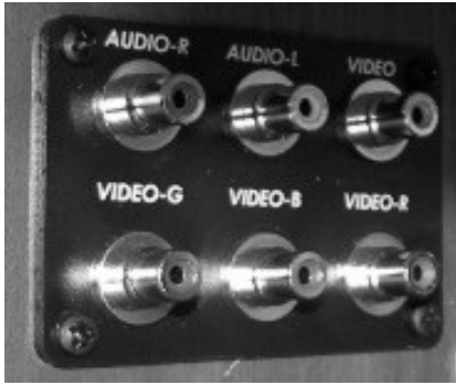
High Definition Audio Video Connection Plate (Located in cabinet near TV) -Typical View
