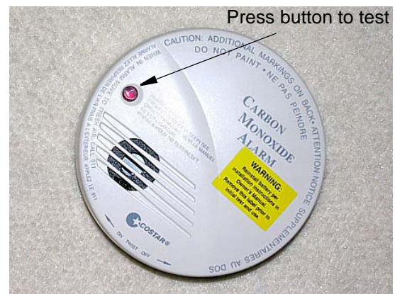
Carbon Monoxide Alarm
