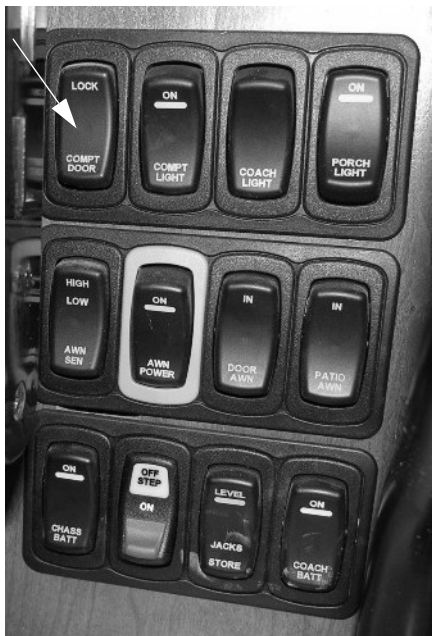
Power Door Locks - Compartment Doors (Located on entry switch panel) -Typical View
