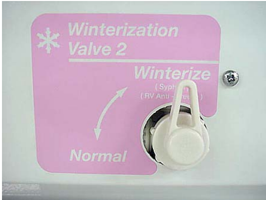
Winterization Valve 2 (Located near water pump)
