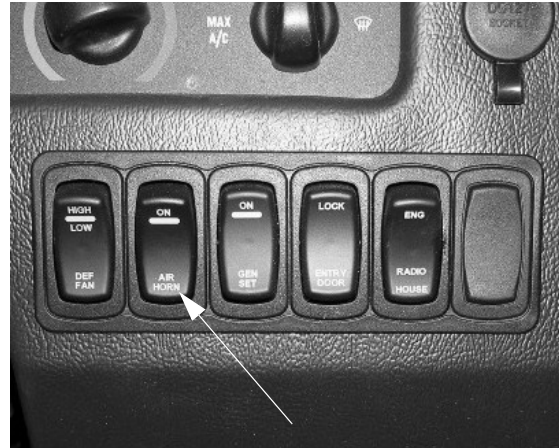
Air Horn Switch (Located on dash or driver side trim panel) -Typical View
