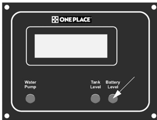
Battery Level Switch
