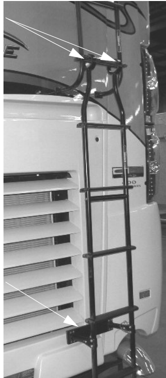
Ladder Extension -Typical View
