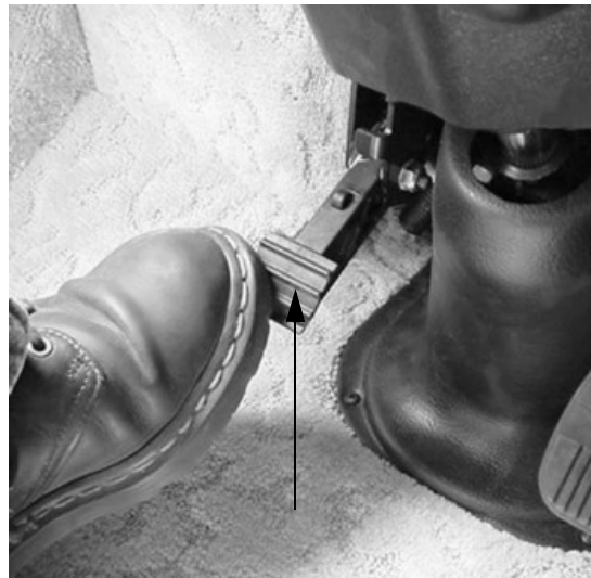
Press pedal to adjust steering wheel tilt or telescope
