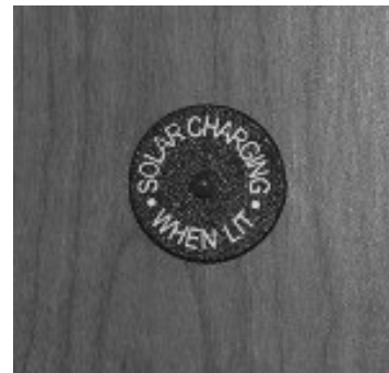
Solar Charging Indicator (Located near monitor panel)
