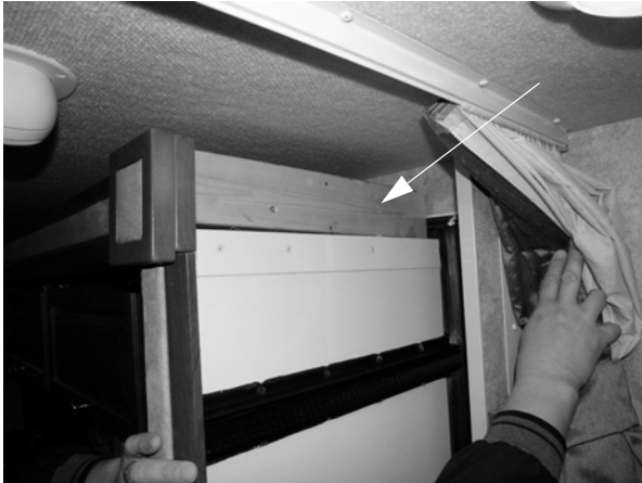
Slideout Travel Support -Typical installation shown
