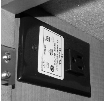
Front TV Ignition Switch Interlock -Typical View
