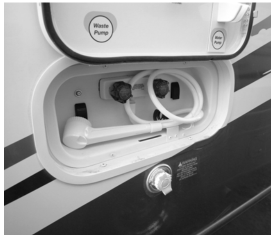
Exterior Shower/Wash Station -Typical View
