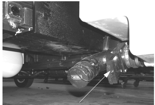
Black Waste Tank Drain Valve (Located beneath coach on mid-driver side) -Typical View
