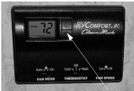
Temp Selector • Press up or down to select temperature
