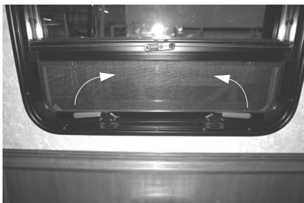
Escape Window (Lift latch handles upward to open)
