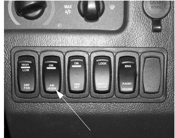
Air Horn Switch (Located on dash or driver side trim panel) -Typical View
