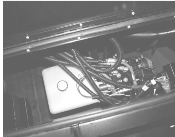
Hydraulic Oil Reservoir (Located beneath entrance step) -Typical View
