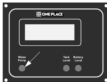
Water Pump Switch (Located on monitor panel) -Typical View
