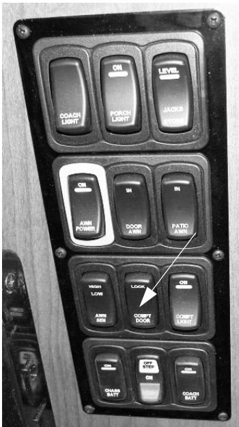
Power Door Locks - Compartment Doors (Located on entry switch panel) -Typical View
