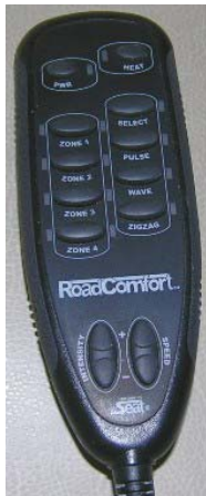
Luxury Cab Seat Remote Control (Located on inboard side of driver and co-pilot seats)
