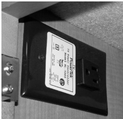
Front TV Ignition Switch Interlock –Typical View
