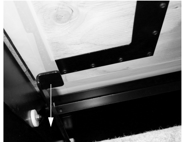
Emergency Retract Lever (Located underneath stepwell cover) • Press DOWN for stepwell cover to store
