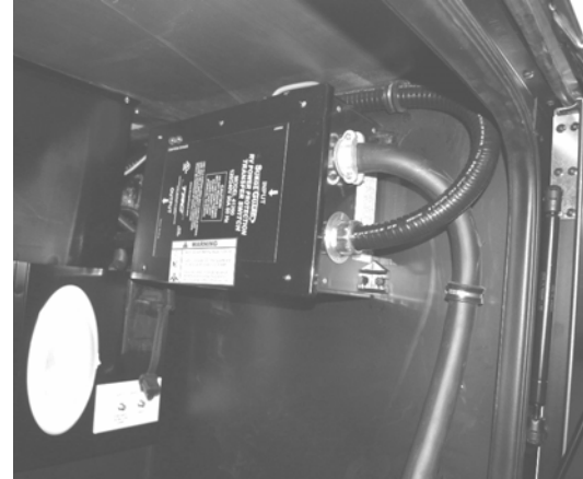
Automatic Power Transfer Box (Located inside or behind utility compartment) -Typical installation shown
