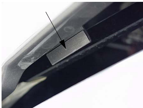
Hood Latch (Squeeze or Pull toward Hood Panel and raise up into open position)
