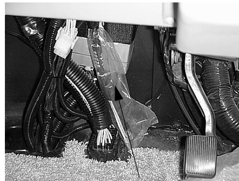
CB Power Wires (in plastic sheath)
