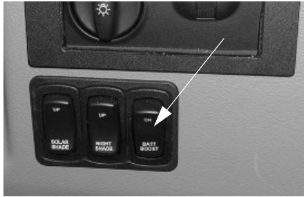
Battery Boost Switch (Located on dash)
