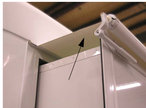
Slideout Cover-Awning -Typical View
