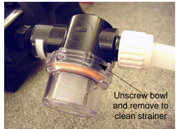
Water Pump Strainer -Typical View
