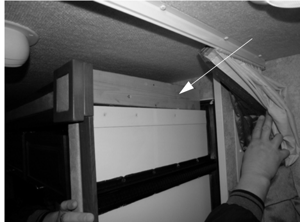
Slideout Travel Support -Typical installation shown
