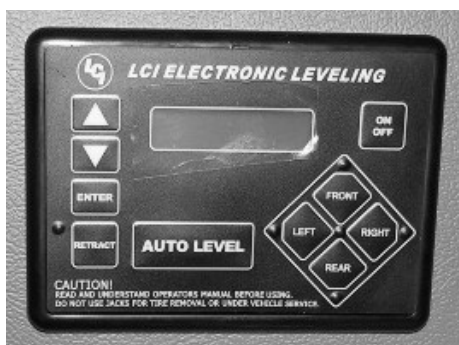
Leveling System Control Panel (Located on dash)
