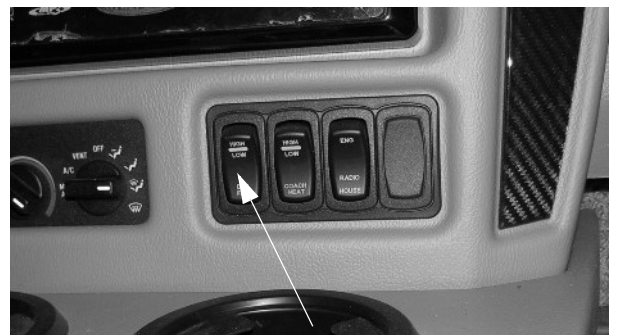
Defrost Fan Switch -Typical View
