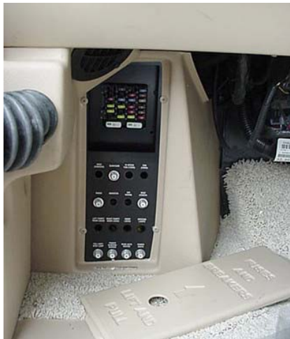
Automotive 12-Volt Circuit Breakers and Fuses (Located beneath left end of dash) -Typical View
