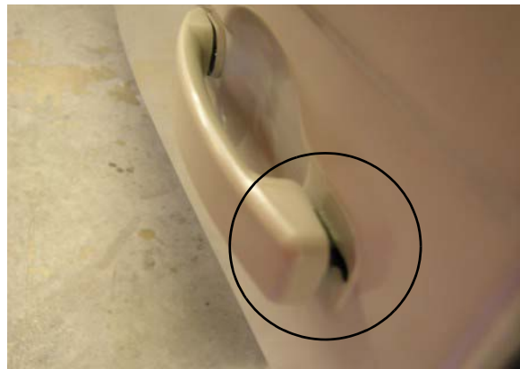
Door Unlatched (note gap)
