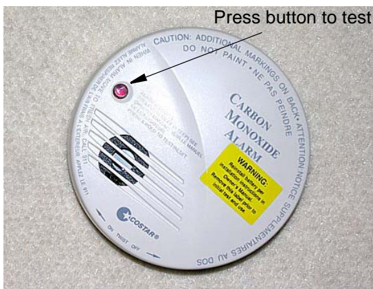
Carbon Monoxide Alarm
