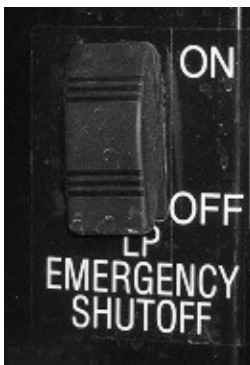
Main Tank Shutoff Switch (Located in driver side compartment) -Typical View
