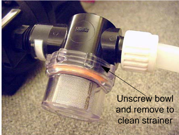
Water Pump Strainer -Typical View
