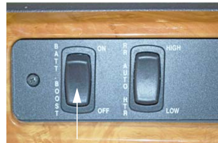
Battery Boost Switch
