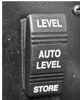
Auto Level Remote Switch (Located near entrance door) -Typical View
