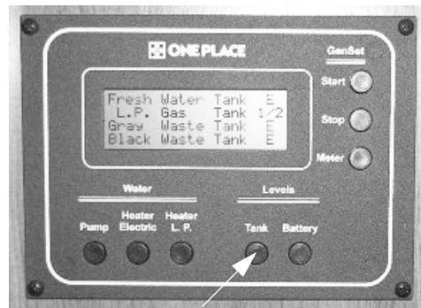
Tank Levels Switch
