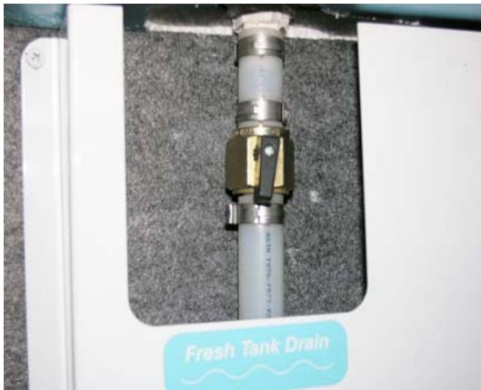
Water Tank Drain Valve -Typical Installation
