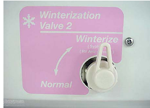
Winterization Valve 2 (See the “Water System Drain Valve Locations” chart at the end of this section for location on your coach)
