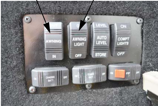
Awning Control Switch and Awning Light Switch (Located near entrance door) -Typical View
