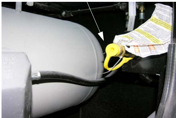
LP Accessory Connection (Located behind LP Tank access door on passenger side of coach) -Typical View
