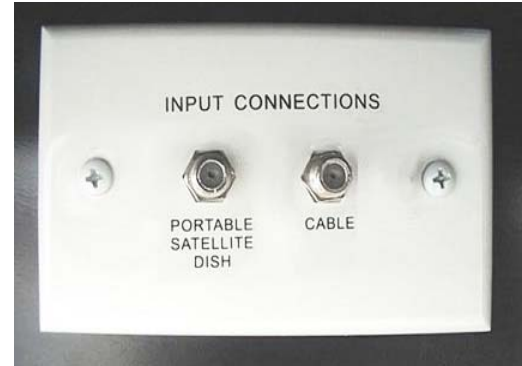
Exterior Connection for Satellite Dish and Cable TV (Located in utility compartment) -Typical View
