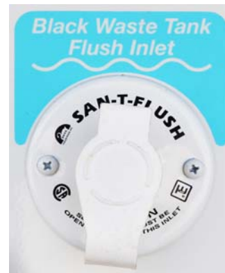
Black Waste Tank Flush Inlet (Located in water service center) -Typical View
