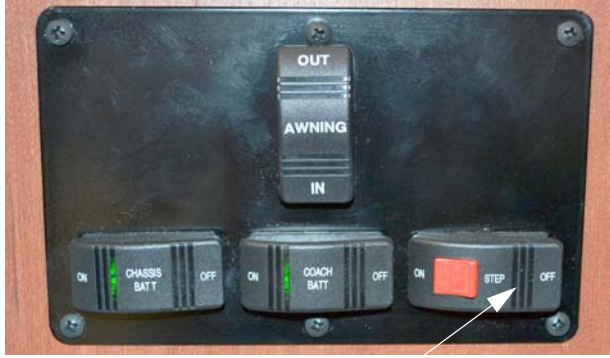
Entry Step Switch (Located near entrance door) -Typical View
