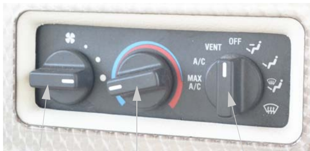
Blower Control Temp Control Mode Selector
