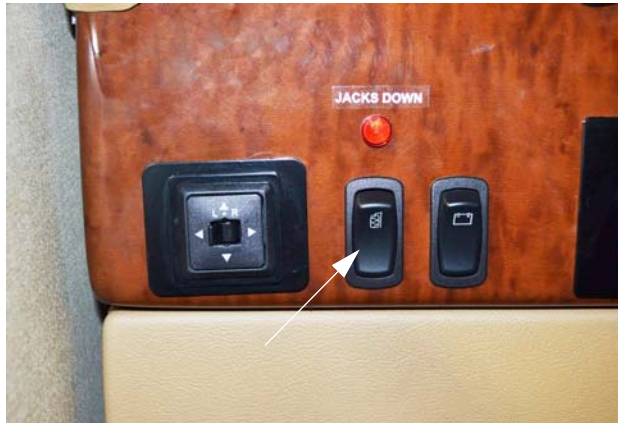
Mirror Heat Switch (Located on dash) -Typical View
