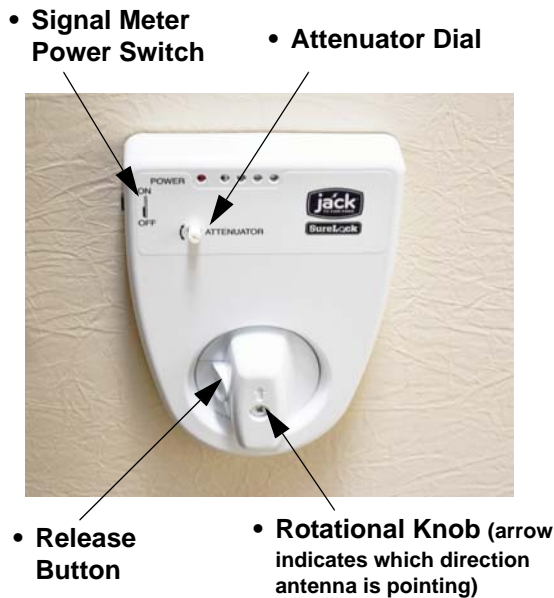
Digital Antenna Signal Meter (Located on ceiling)
