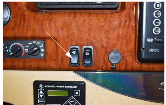
Defrost Fan Switch (Located on dash) -Typical View
