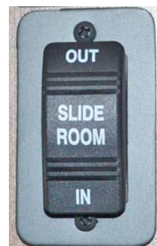
Slideout Switch (Your coach may have one or more slideout switches depending on model, options, and available equipment) -Typical View
