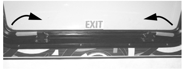
Escape Window (Lift both latch handles upward and push window open) -Typical View
