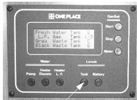
Tank Levels Switch
