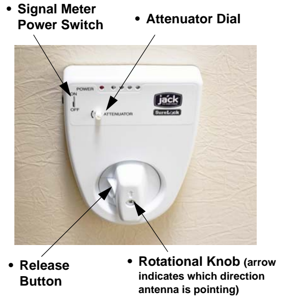
Digital Antenna Signal Meter (Located on ceiling)
