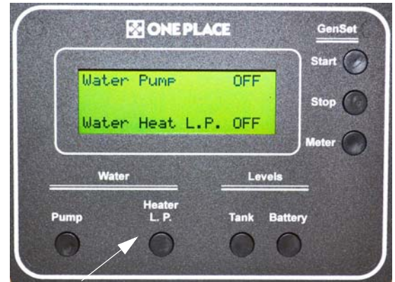
Propane Gas Water Heater Switch (Located on OnePlace® monitor panel)
