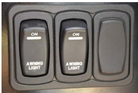
Awning Light Switches (Located near entrance door) -Typical View
