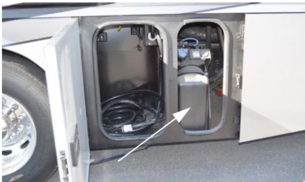
Diesel Exhaust Fluid Fill Tank (Located in driver side compartment behind rear wheel) -Typical View
