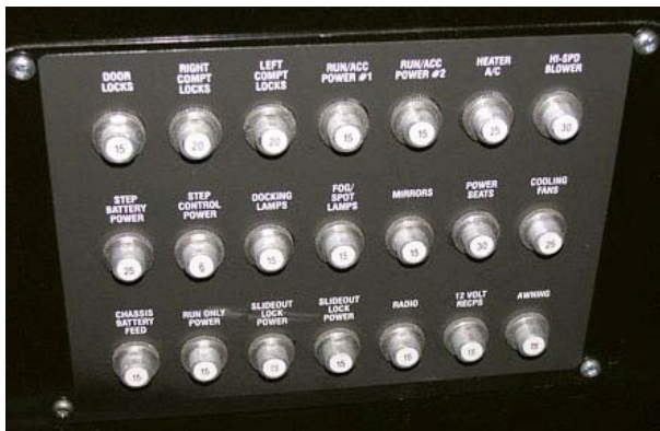
Automotive Circuit Breakers (push to reset)
