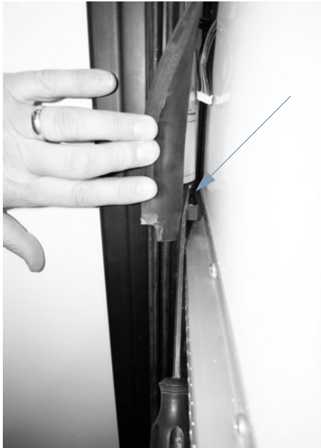
Slideout Motor (Located behind slideout wipe seal)
