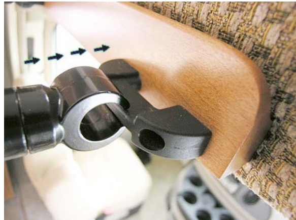
Attaching Bunk Ladder
