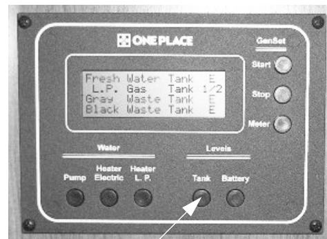
Tank Levels Switch
