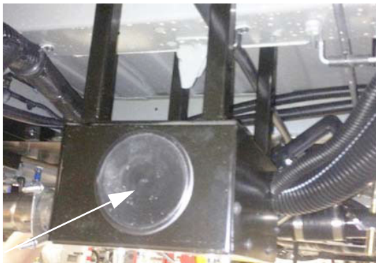
Waste Pump Enclosure (Located beneath motorhome)
