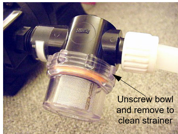
Water Pump Strainer -Typical View
