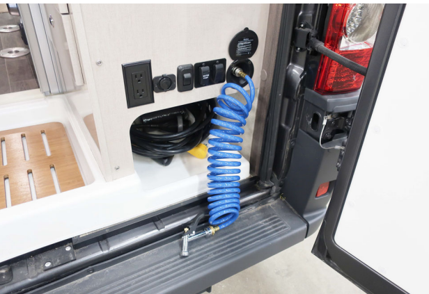
Exterior Shower/Wash Station (located behind rear passenger side door) *Model 59K shown
