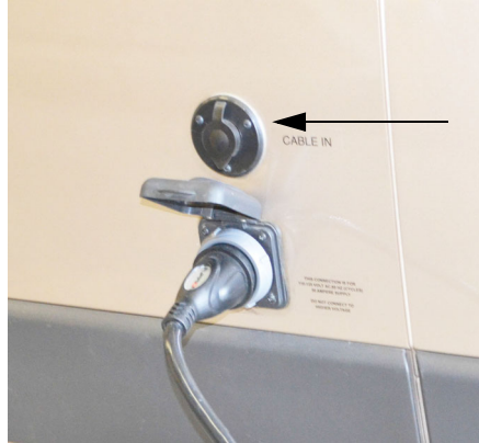
Cable TV Input Connection (Located on the left sidewall) *Model 59G shown
