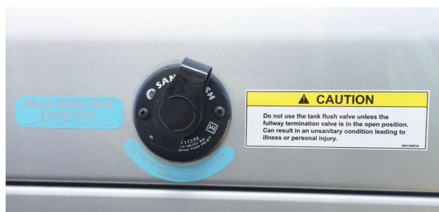
Black Waste Tank Flush Inlet (Located on left sidewall)
