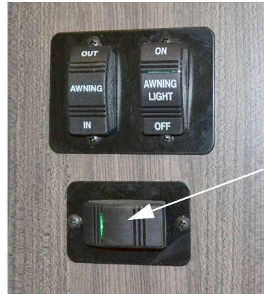
Accent LED Running Board Light Switch (Located near sliding door) -Typical View
