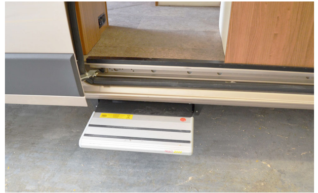
Entry Step (Located near sliding door) -Typical View (Extended position shown)
