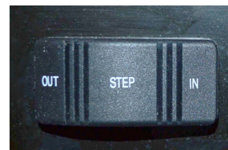
Entry Step Switch (Located near sliding door)
