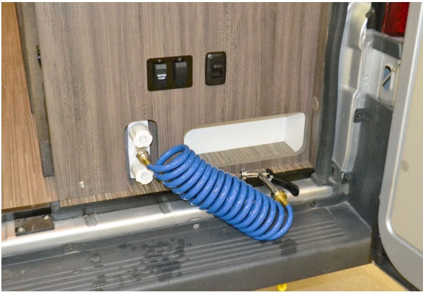
Exterior Shower/Wash Station (located behind rear passenger side door) *Model 59G shown
