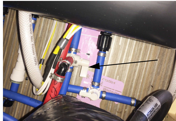
Winterization Valve 1 (Water Heater Bypass Valve) (See “Water System Drain Valve Locations” chart at the end of this section for location on your model) *Model 59K shown
