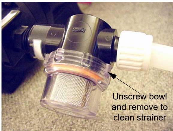
Water Pump Strainer -Typical View
