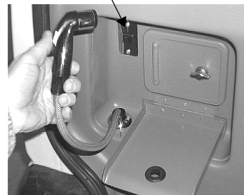
Water Pump Switch
