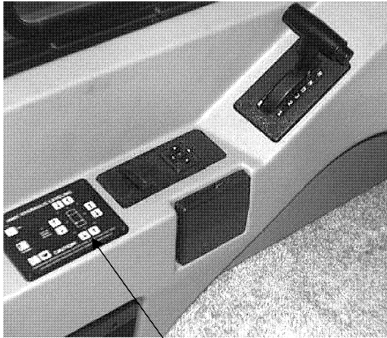
Leveling System Control Panel
