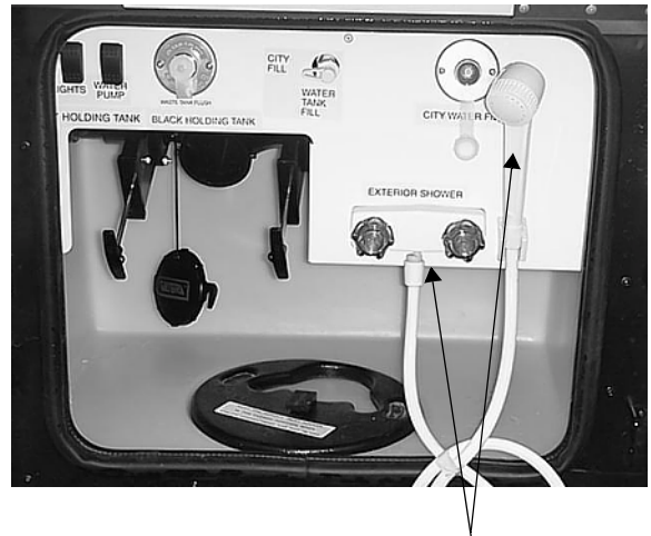
Exterior Shower/Wash Station
