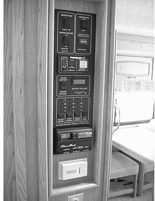
One Place Monitor Panel
