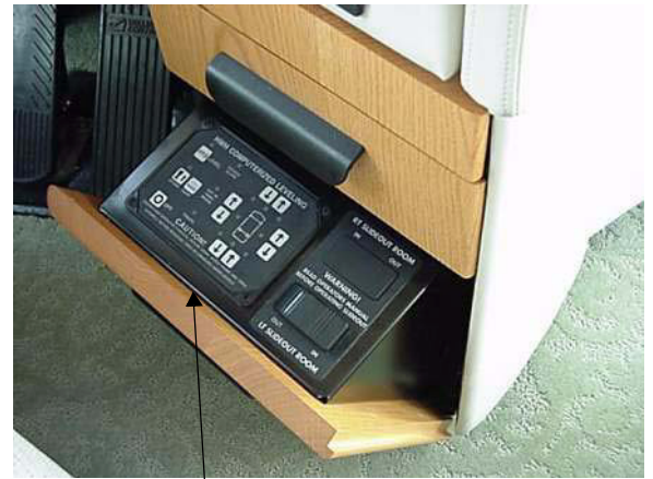
Automatic Leveling System Control Panel
