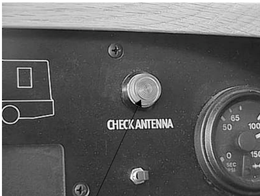
“Check Antenna” Light
