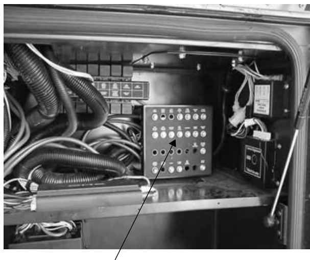
Automotive 12-Volt Breaker Panel
