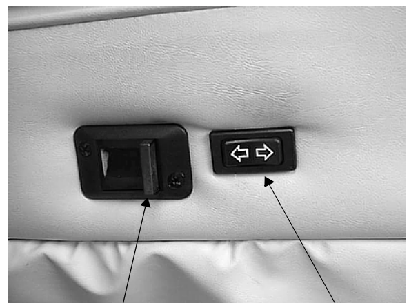
Push Lever to Recline Seat Press Button for Lumbar Support ← Less - More →
