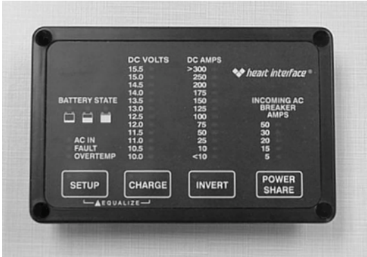
Inverter Charger Control Panel
