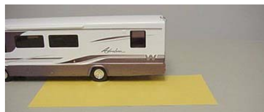
Weighing Left Rear 'Corner'
