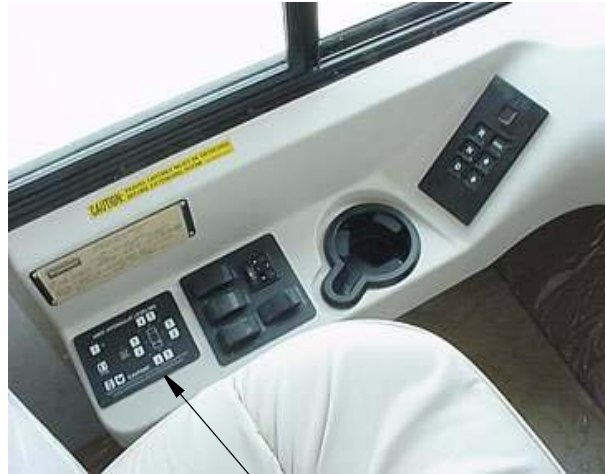
Leveling System Control Panel
