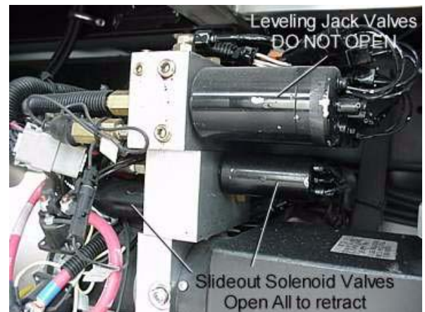
Leveling/Slideout System Hydraulic Pump (Note valve positions in relation to fluid reservoir)
