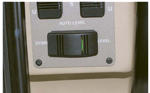
Auto Level Switch inside Entrance Door
