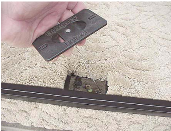
Pull chain to release step mechanism and manually slide step cover back.
