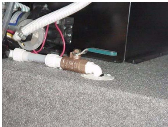
Water Line Drain Valve in RH Exterior Water Pump Compartment All Models
