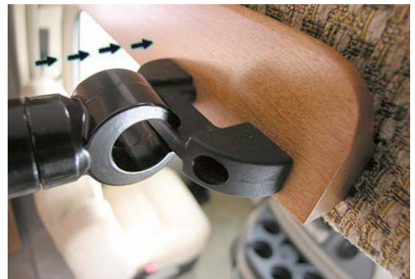
Attaching Bunk Ladder
