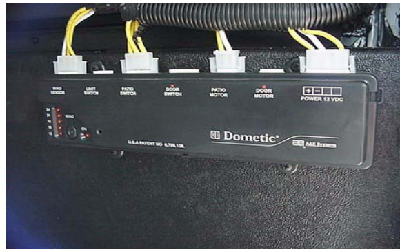
Awning Control Box (located in exterior compartment)
