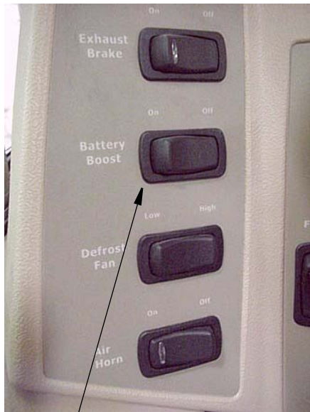
Battery Boost Switch
