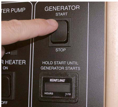
Generator Switch and Hourmeter on monitor panel
