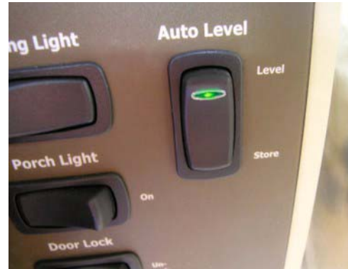
Auto Level Switch inside Entrance Door
