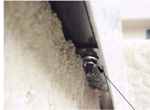
Hydraulic Pump Access - remove nut from bolt on underside of step and lift off step
