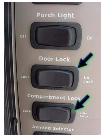
Power Door Locks on entry switch panel
