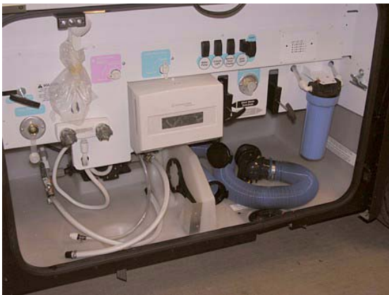
Water Service Center - typical view
