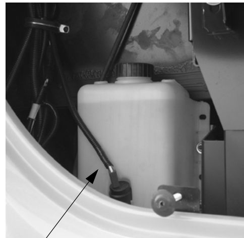
Windshield Washer Reservoir (behind front hood panel)
