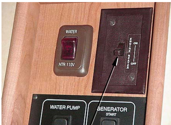
Diesel Engine Heater Switch (Typical)
