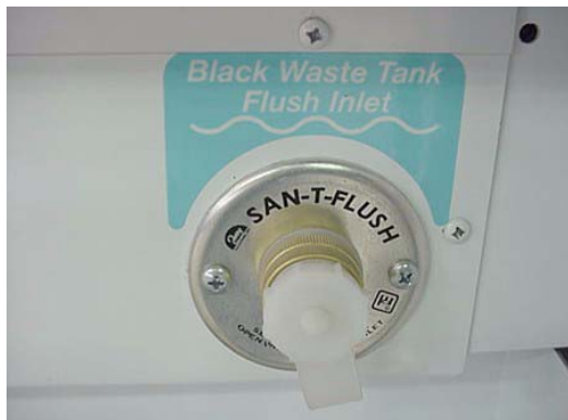
Water Tank Flush Inlet (typical)
