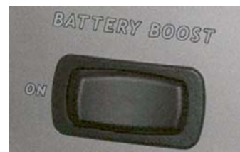
Battery Boost Switch
