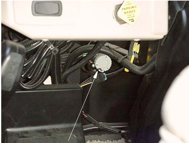
Diagnostic plug on steering column support beneath left side of dash
