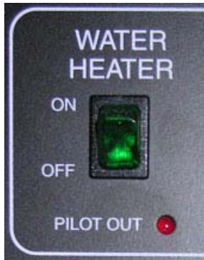
Gas Water Heater Switch on systems monitor panel
