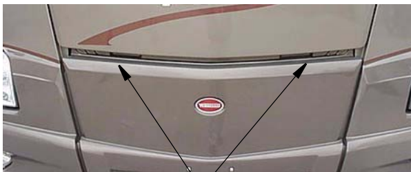
Squeeze both latches then pull the hood panel outward and swing it up to open.
