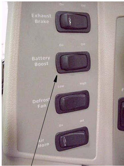
Battery Boost Switch
