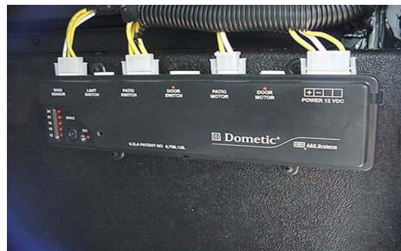
Awning Control Box (located in exterior compartment)
