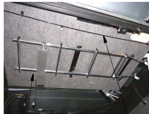
Roof Ladder Extension
