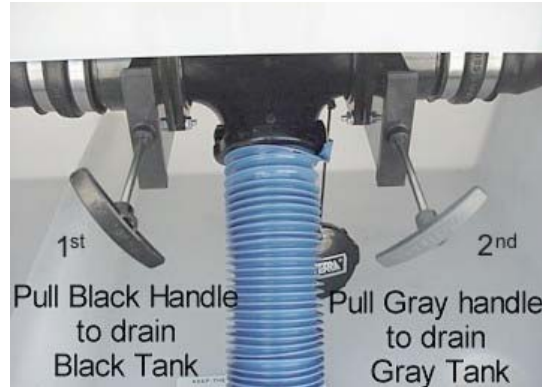
Holding Tank Dump Valves (Typical)
