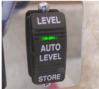
Auto Level Switch (Located inside entrance door)
