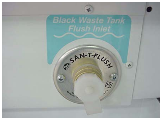
Water Tank Flush Inlet (typical)
