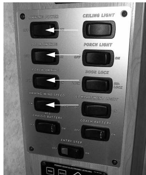
Awning Control Switches - Typical View (Located near entrance door) -Model M39N shown
