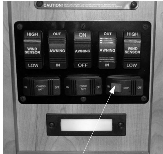
Red Activation Lever The red Activation Lever located on the entry step switch must be depressed in order to put the step switch in the ON position.
